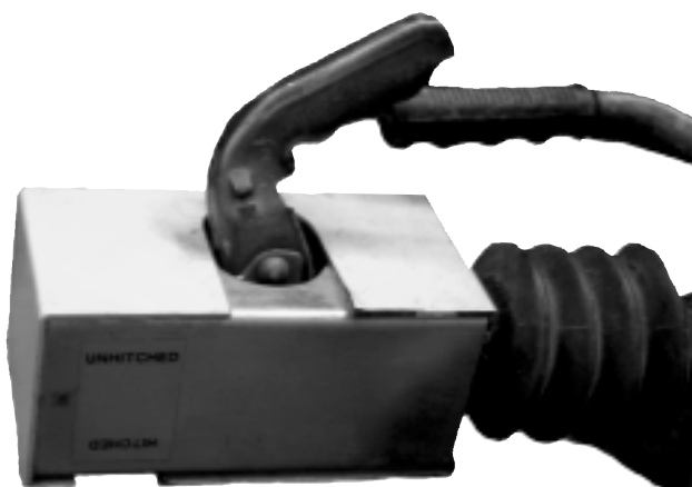
The hitchbox encloses the coupling head and bolts and can be used also while the vehicle is attached.
