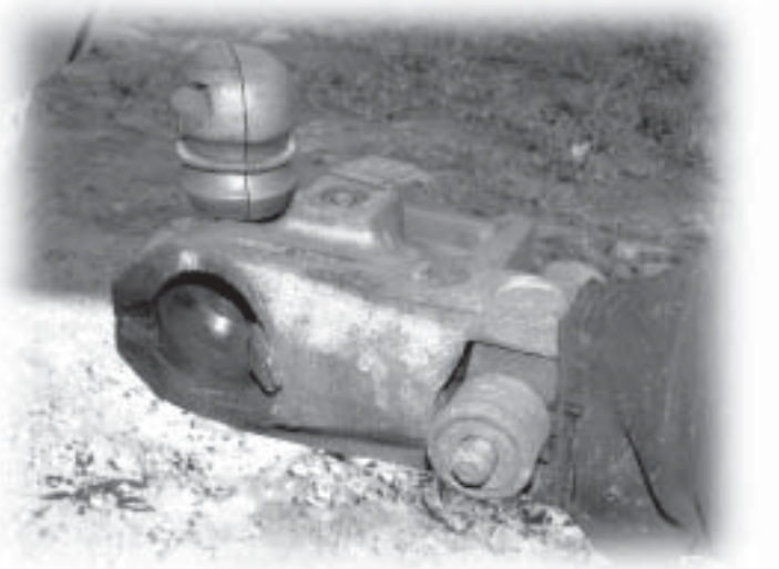
The expandable hitchlock is seen here sitting on the Bradley triple lock, which has an in-built coupling head lock and shear bolts to prevent the coupling head being unbolted
