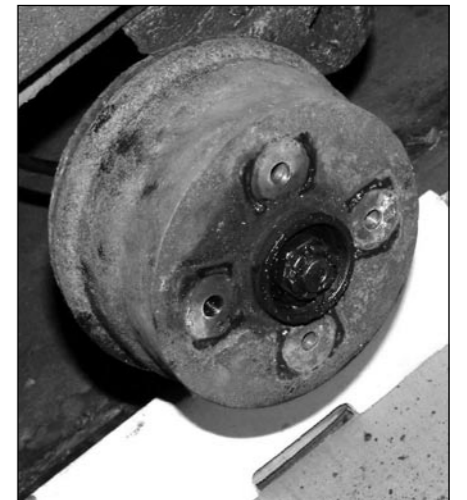
BRAKE DRUM: Grease cap removed
